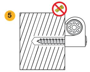
For concrete and tile: screw directly into 4 mm hole – no plug required.
