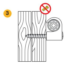
For wood, fibreboard and plywood: screw **directly** into material - no plug required.
