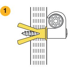
For 13 mm single-layer plasterboard: mount using yellow plug (KP yellow).
