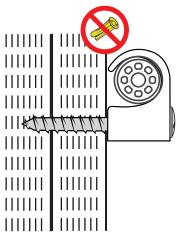
For double-layer plasterboard – no plug required. If screw "goes over", mount using yellow plug (KP yellow) in the created hole.
