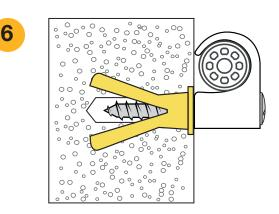
For aerated concrete: mount using yellow plug (KP yellow). For densities above 600, screw directly into material.
