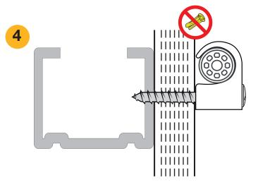
For 13 mm single-layer plasterboard on metal profile – no plug required.
